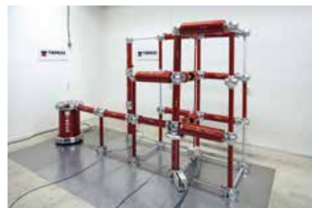
3-stage DC Voltage Test Set-up
