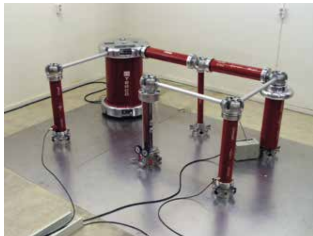
Measurement of flashover voltage in vacuum and under pressure
